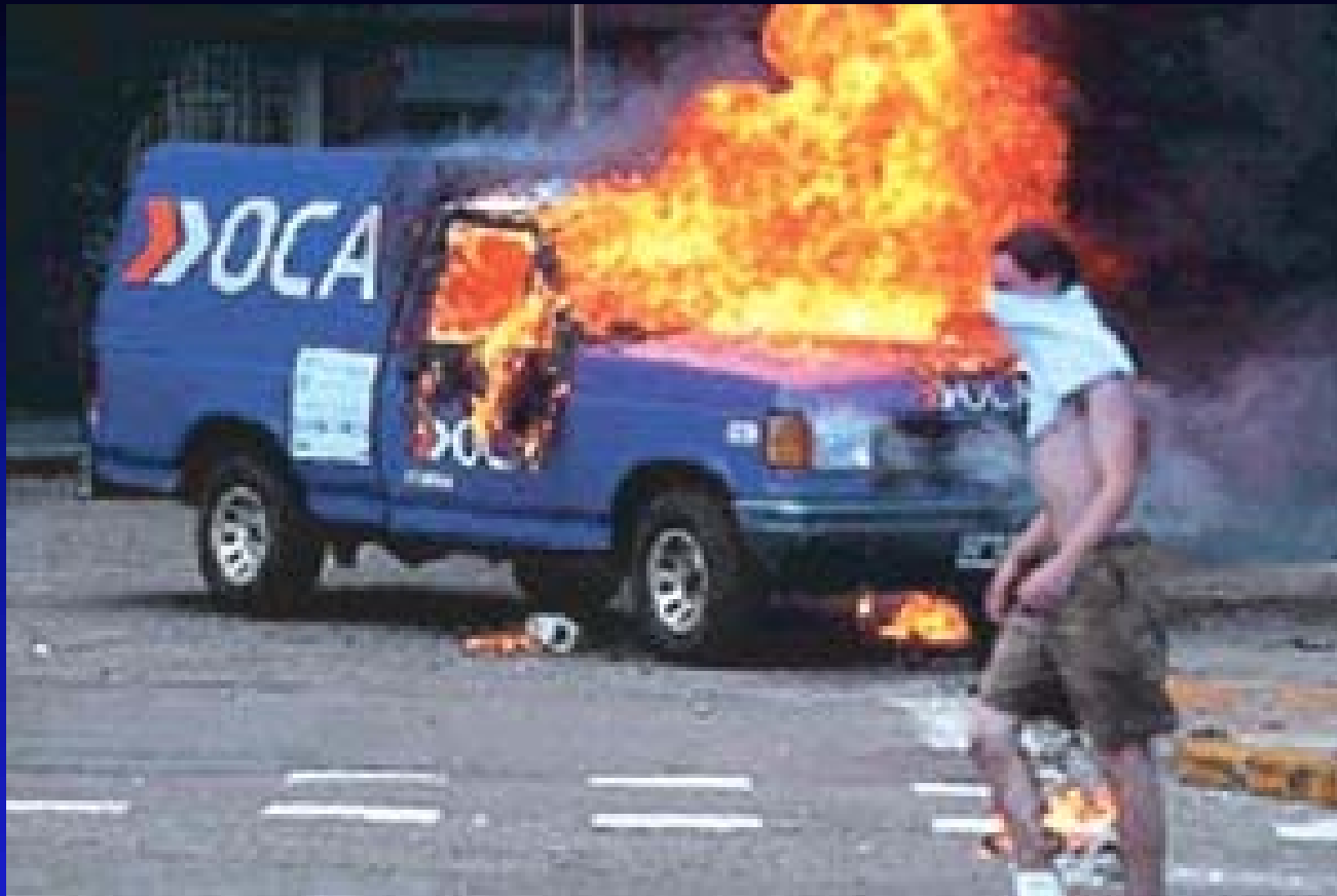
Natural Gas Pick-Up, on fire after riots, Dec.20 2001 (fire was produced by a Molotov cocktail; there was no explosion at all)
